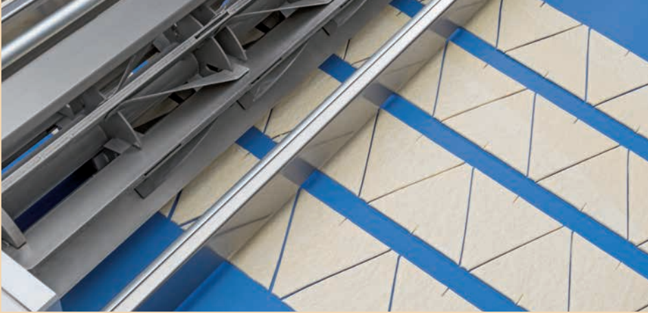
The triangles can be cut with a rotary cutting shaft or stamped with a guillotine from the dough band.
