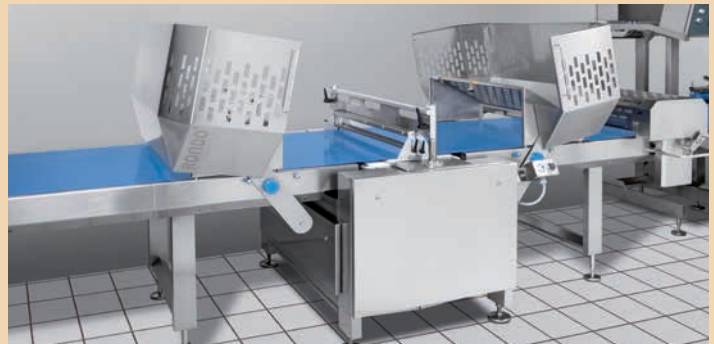
Easy accessibility of the guillotine in ASTec design enables easy cleaning.
