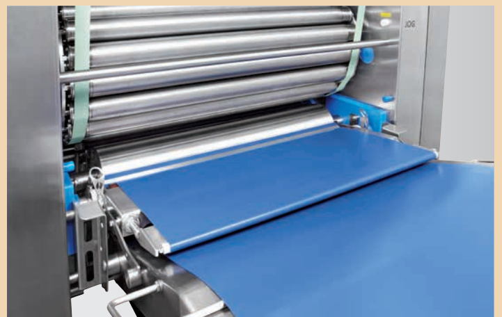
Large satellite heads with two lower rollers treat the dough band particularly gently.
