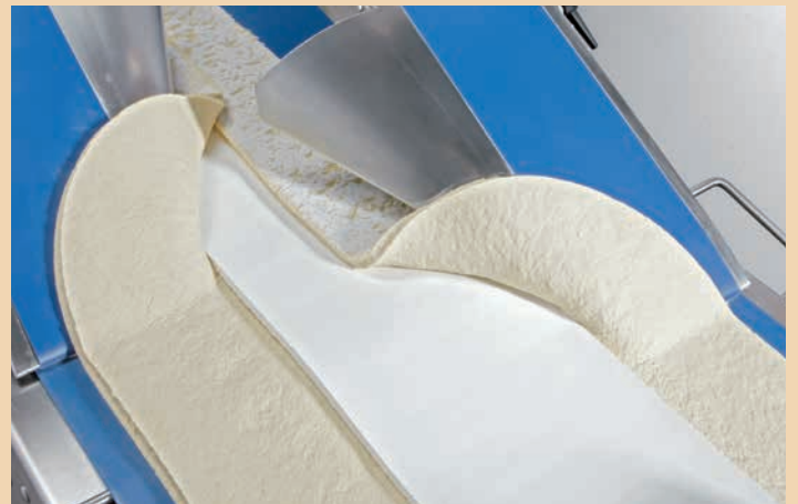
A homogeneous dough band and a consistent layer of fat are the basis for the high quality of the dough band.
