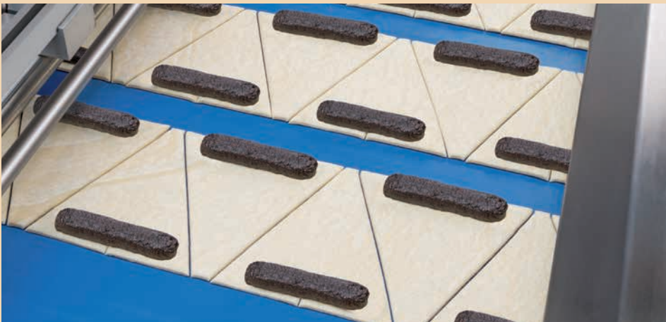
For filled croissants, you can apply the filling either in the middle or along the base.
