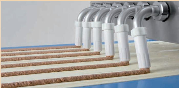
No matter whether cream, vegetable or meat fillings are involved, RONDO filling devices deposit them without difficulty.
