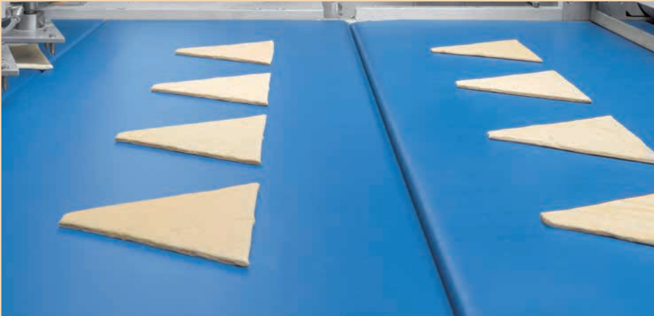
High-speed rotating devices controlled by servo motors turn the triangles into the exact position.
