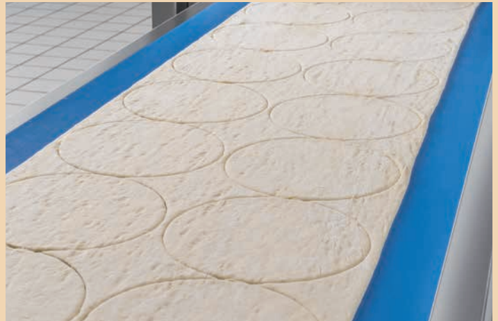
A dough band without stress is the requirement in order that pizzas stay round.
