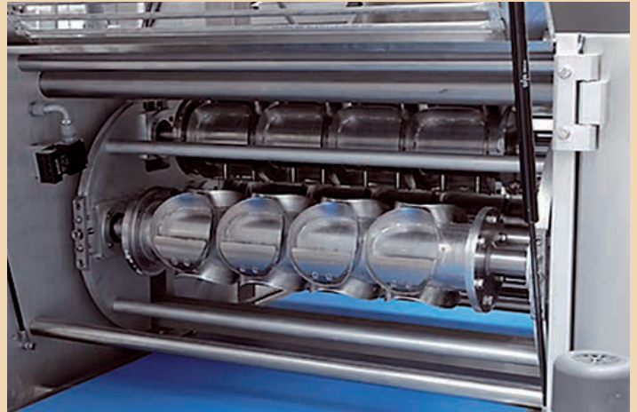
Product changes are very simple, using a revolving cutting station, for example.
